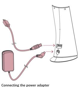
Connect power adapter input into power socket
