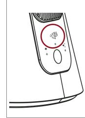
Lightly press the fan switch to turn on the air purifier. There are three speed settings (low, medium and high).
