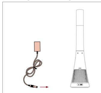
Plug the power adaptor into the light, and into a standard household 100V - 240V power outlet.
